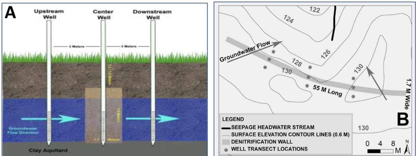
(A) A side-view and (B) an overhead view of the wall indicating the hydrology. In this case the wall is installed down to a clay layer and approximately perpendicular to the groundwater flow direction.
