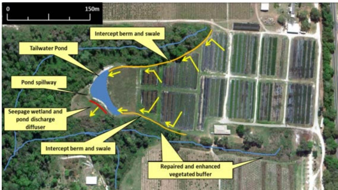
BMP modifications added to address surface runoff from overhead irrigation area. Post implementation overland flow is intercepted by berms and directed via swales to a tailwater pond. Water detained in the pond is released at a controlled rate to a seepage wetland and eventually flows back to the tributary.
