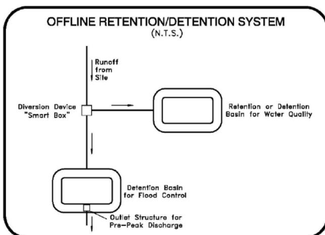
Off-line retention/detention systems provide an off-line retention pond for the treatment volume and an on-line detention pond for flood control and attenuation of peak discharges. A diversion device, often called a "smart box", is used to divert first-flush stormwater runoff into the retention pond. When the retention pond fills, the remaining stormwater runoff is diverted directly to a detention pond for flow attenuation purposes.
