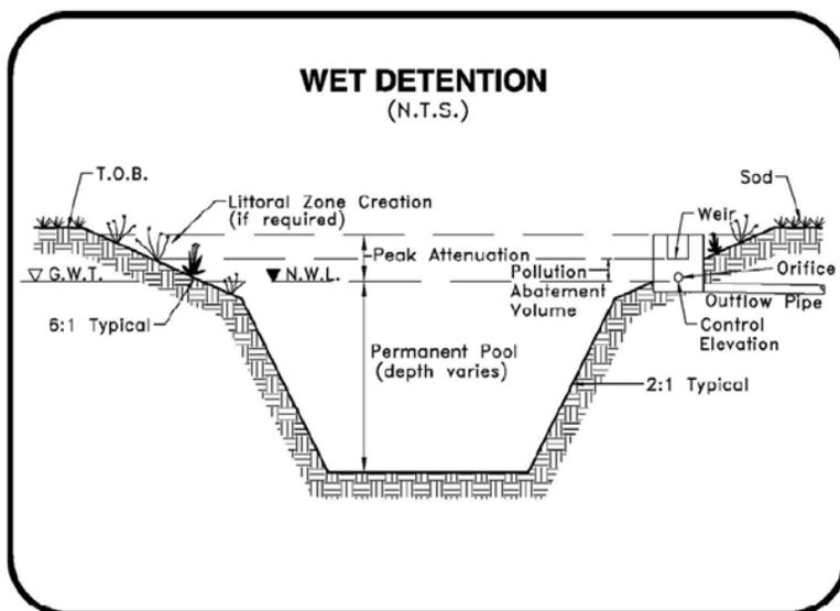
Wet detention systems are currently a very popular stormwater management technique throughout the State of Florida, particularly in areas with high groundwater tables. A wet detention pond is simply a modified detention facility which is designed to include a permanent pool of water. These permanently wet ponds are designed to slowly release collected runoff through an outlet structure.
